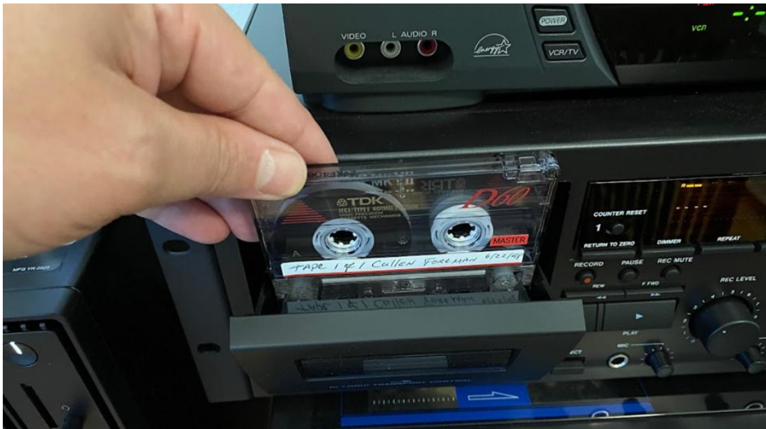
Figure 7: The broad side of the cassette goes in first.
