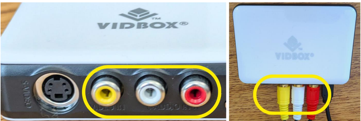
Figure 7: Match the colors when plugging the RCA cables into the Vidbox.
