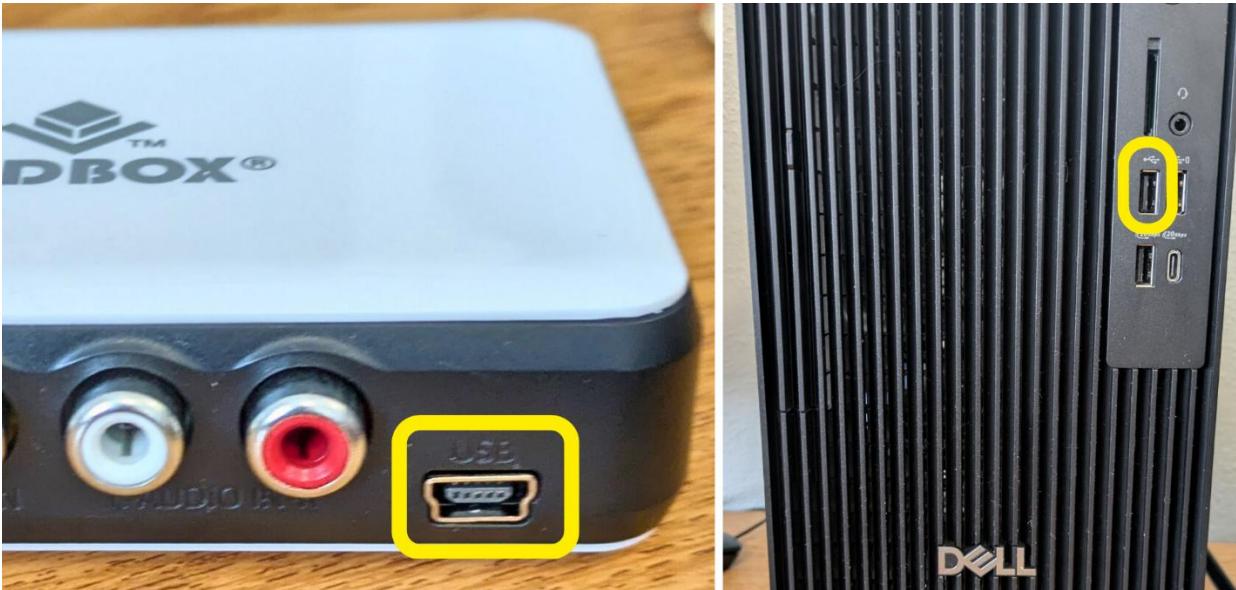
Figure 6: Connect the USB cable to ports on the Vidbox unit and computer.
