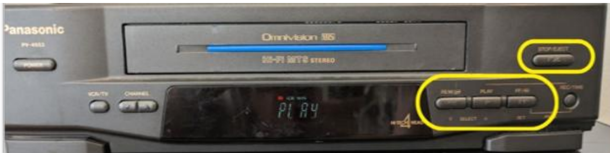
Figure 16: Playback controls on the VHS player.
