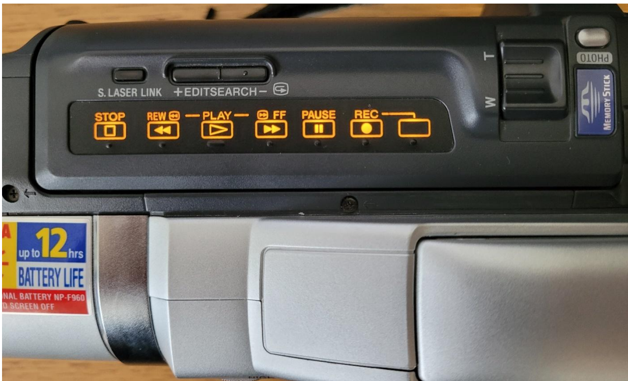
Figure 20: Playback controls on the top of the camcorder.
