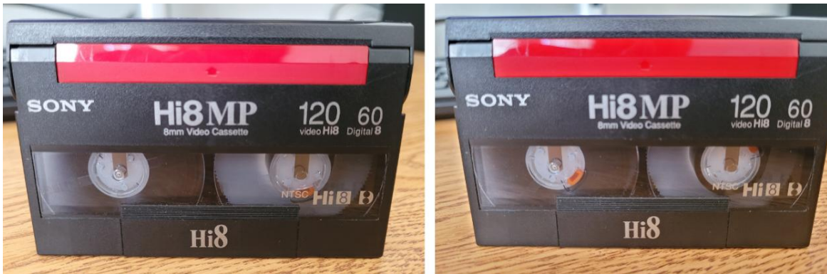
Figure 9: Cassette on the left is fully rewound; cassette on the right is only partially rewound.
