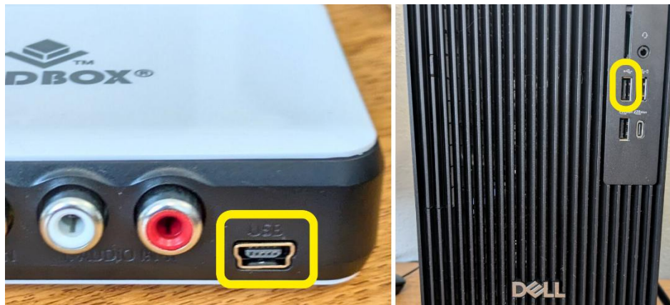
Figure 6: Connect the USB cable to ports on the Vidbox unit and computer.
