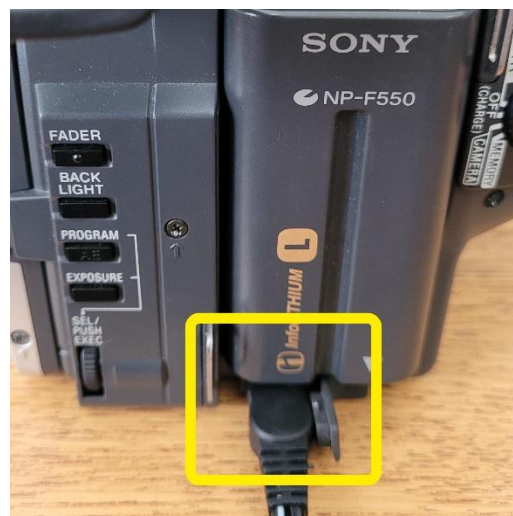
Figure 10: The power cord inserted into the camcorder port.
