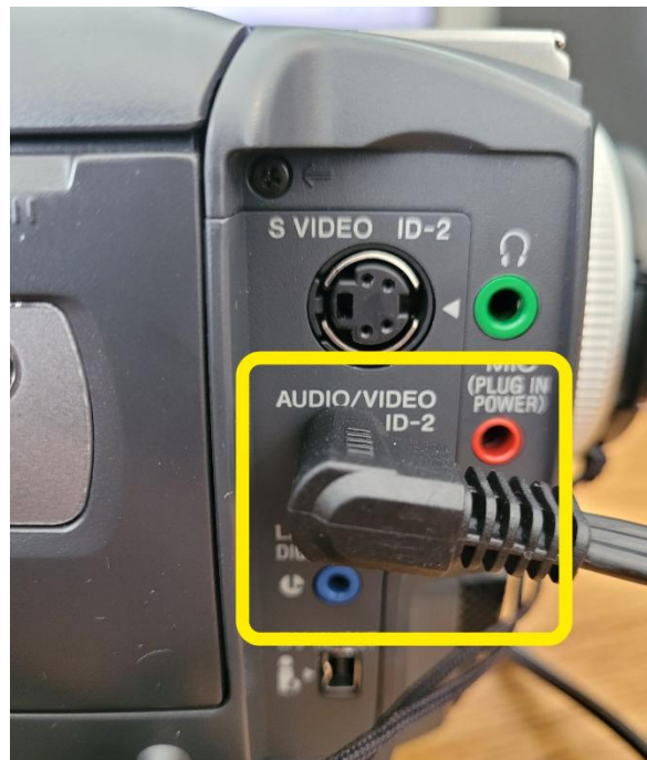
Figure 8: Plug the jack connector into the camcorder's Audio/Video ID-2 port.
