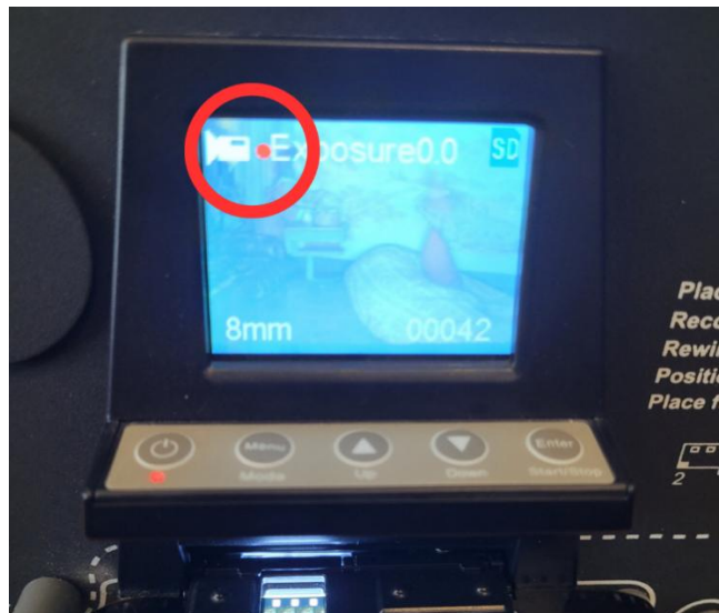
Figure 16: A red dot indicates recording is in progress.
