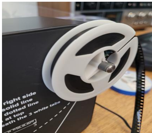
Figure 19: Reel positioned to rewind (note position of the film sprocket holes).
