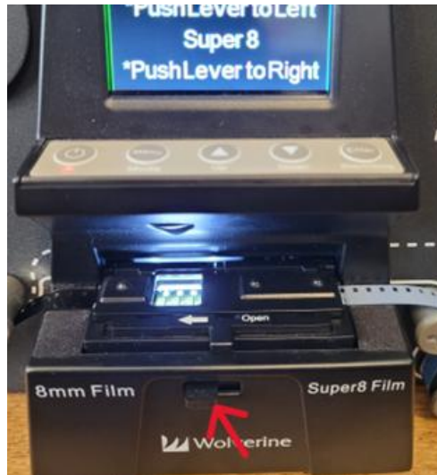
Figure 15: Lever to switch between 8mm and Super 8.
