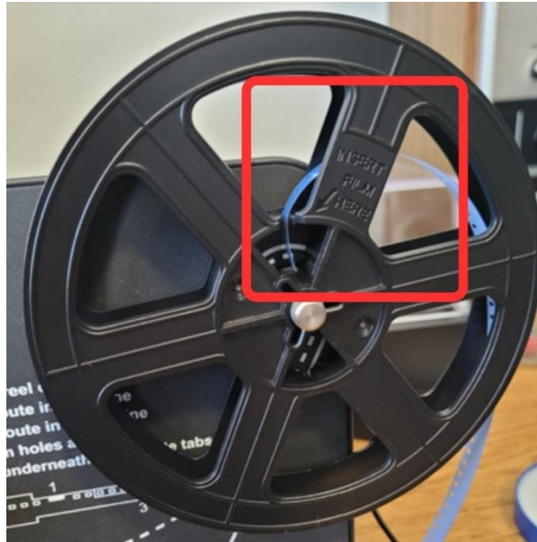
Figure 11: Film inserted in slot on empty take-up reel.
