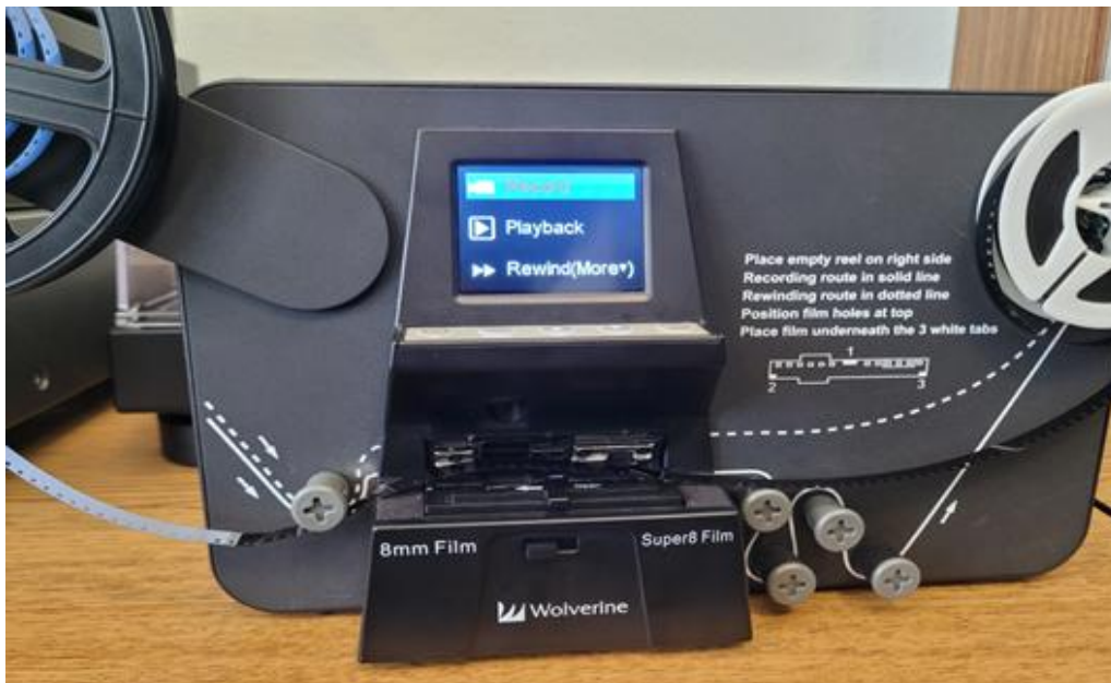
Figure 21: Follow the dashed white line diagram for rewinding.
