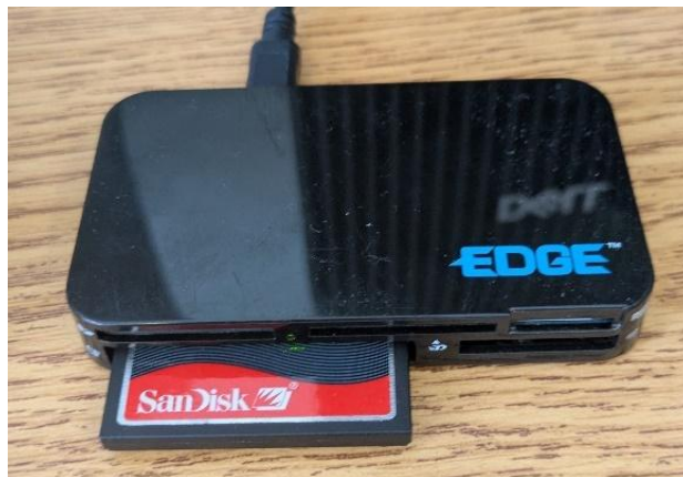
Figure 5: Flash card properly installed.
